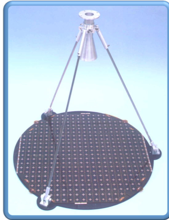
Integrative design of RA & solar panels
