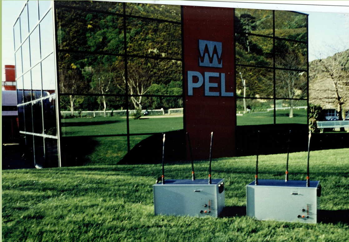
Single user N=3 MIMO at 450MHz. (PEL, New Zealand, 1987)
